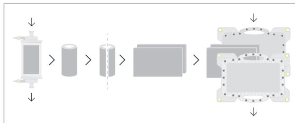
Figure 2b: Design for the cassette is derived from the capsule by cutting and creating two membrane stacks.
