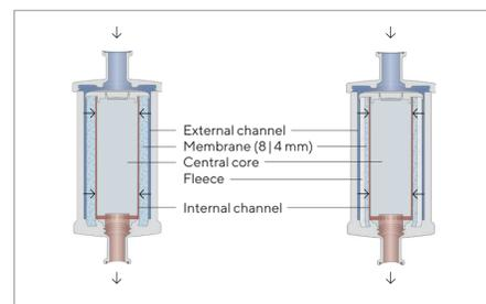
Figure 5: Design and flow path of membrane adsorber capsules with 8 mm (left) and 4 mm (right) bed height.
