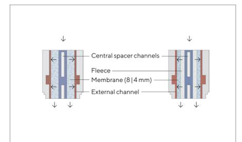
Figure 6: Design and flow path of the scalable cassette format with 8 mm (left) and 4 mm (right) bed height.
