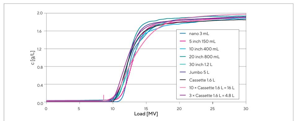
Figure 7: BSA breakthrough curves of capsules and single, 3 × 1.6 L cassette and 10 × 1.6 L cassette, 8 mm bed height versions.
