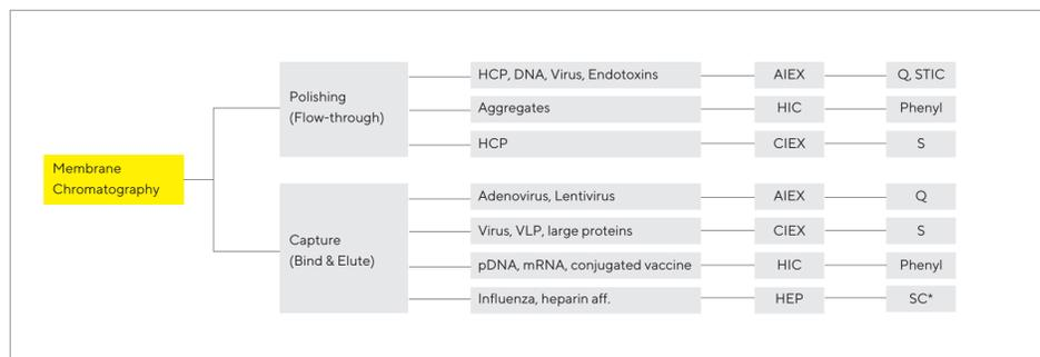
Figure 1: Typical modes of operations and applications for membrane adsorbers in the biopharmaceutical industry. Ligands: S = sulfonic acid for cation exchange (CIEX), Phenyl as hydrophobic interaction chromatography ligand (HIC), Q = quaternary ammonium, STIC = STIC PA primary amine (salt tolerant) for anion exchange (AIEX), SC = sulfated cellulose (\*) prototype, heparine pseudo affinity (HEP)
