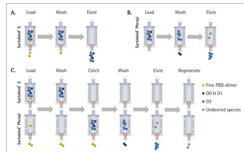
**Figure 1:** Process diagram. (A) Bind | Elute using Sartobind<sup>®</sup> S to remove residual payload, and (B) Bind | Elute using Sartobind<sup>®</sup> Phenyl to remove aggregate in stand-alone model; (C) Simplified process to purify target ADC with Sartobind<sup>®</sup> S and Phenyl in tandem model.
