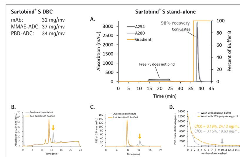
**Figure 2:** (A) Removal of residual PBD using Sartobind<sup>®</sup> S in stand-alone model. The quenched reaction mixture (gram scale) was loaded to a 150 mL Sartobind<sup>®</sup> S membrane, then washed with 10 mv binding buffer prior to elute. (B) HIC and (C) SEC profiles showing the removal of free PBD dimer. (D) LC-MS method showing PBD dimer removal efficiency with Sartobind<sup>®</sup> S.
